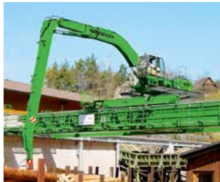
The 16-year-old 835 C-Series model at work in the Finkbeiner KG log yard after 55,000 service hours.
