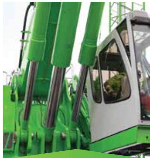
With their large center cylinder set between the boom's two lift cylinders, Green Hybrid machines are easy to distinguish from conventional material handlers.
