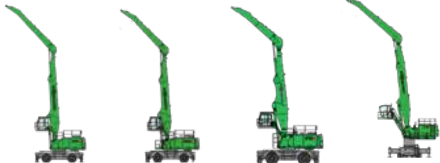
With their large center cylinder set between the boom's two lift cylinders, Green Hybrid machines are easy to distinguish from conventional material handlers.
