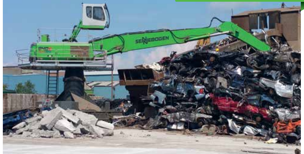
The pedestal-mounted, electric drive 840 material handler at Ferrous Processing & Trading (FPT) takes the worry out of emissions.
