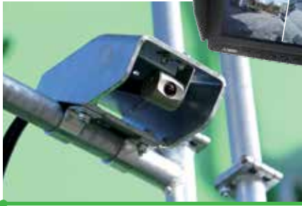
A dual camera system including cab monitor ensures 360° visibility. Only SENNEBOGEN provides a right-view and rear-view camera as standard to provide a view past the boom.
