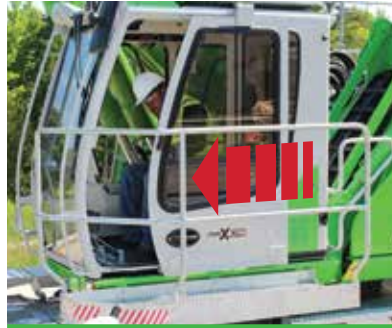
The sliding door of the maXCab allows safer entry and exit than a hinged door.
