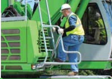
Wide steps, an access ladder and handrail ensure 3-point contact when climbing from the ground to the upper deck.
