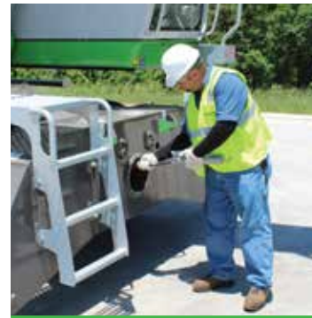
Daily lubrication of the undercarriage at front of machine from ground level.
