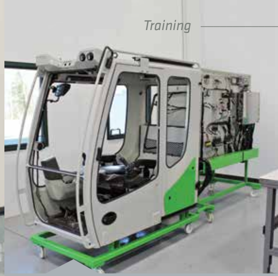
A working mock-up of the operator's station simulates all electrical and hydraulic controls for SENNEBOGEN's maXCab, standardized for all material handler models.
