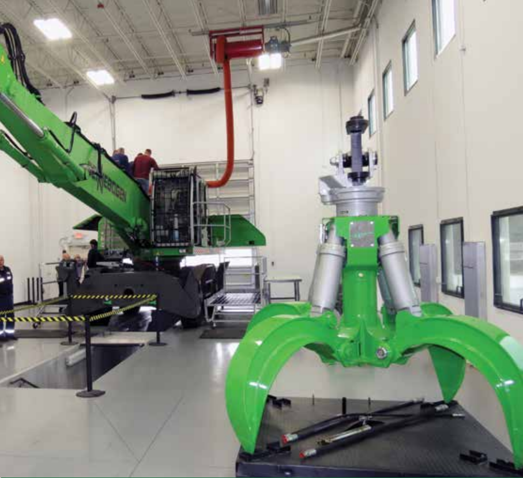
A working mock-up of the operator's station simulates all electrical and hydraulic controls for SENNEBOGEN's maXCab, standardized for all material handler models.
