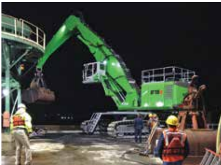
The 875 R-HD model operated by Charleston Bulk Transfer can move material as quickly as the giant 880 R-HD it replaced, but it consumes less than 60% as much diesel fuel.
