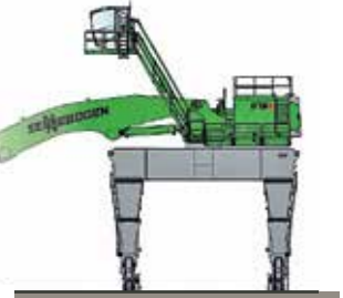
Railway Gantry Undercarriage
