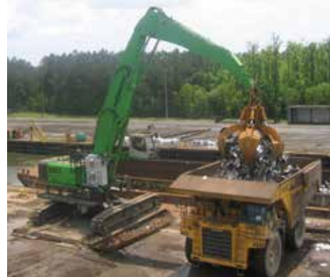
This SENNEBOGEN 880 R-HD electric drive scrap handler in Charleston is moving more material with its 10 yard grapple than the facility's former rope crane produced with a grapple twice the size.
