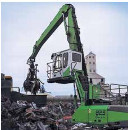
A SENNEBOGEN 825 M D Series with high rise cab gives the CASS operator a clear view.
