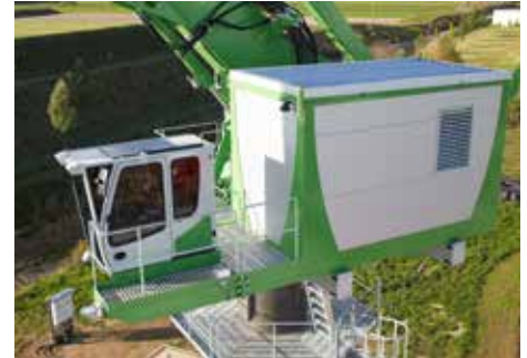
The 8130 EQ machine is equipped with a compact walk-in powerpack that provides easy access to all maintenance check points, all using standard SENNEBOGEN components
