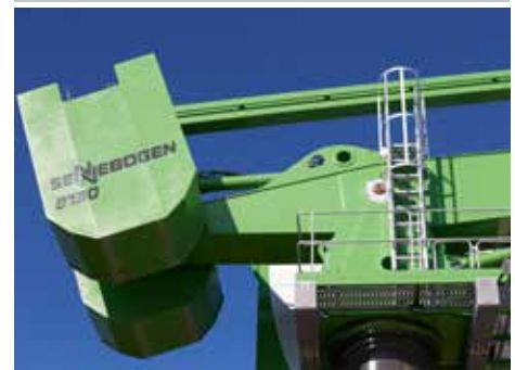
The EQ counterbalance uses a simple lever mechanism to automatically adjust to the movement of the load on the boom.
