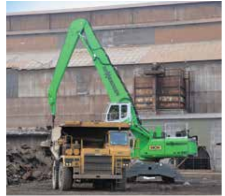
The SENNEBOGEN 850's standard design with guarded catwalks, railings and safety cameras inspired MCM to retrofit its entire equipment fleet to an equal standard.
