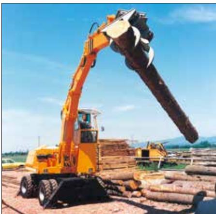
1974: Timber handling machine with elevated cab
