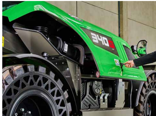
Spacious access to the engine compartment with just one handle. The side plate of the engine nacelle can also be removed.
