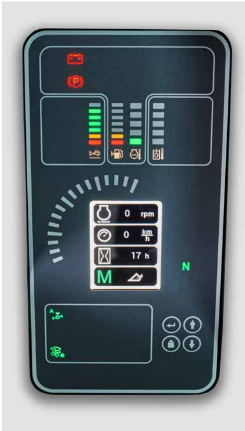
Clear control panel and display console including error code display.
